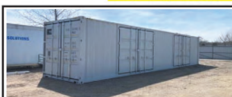
2024 CIMC 40' Shipping container, type TC-S-6101G.1(2) double side doors
