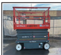
2018 Skyjack SJ111 4632, Work Height: 38', Raised Platform Height: 32'
